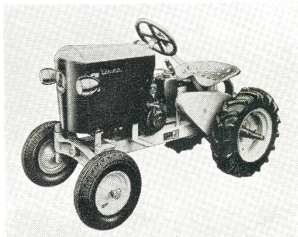
The 1958 Tiger tractor features the Borg-Warner three-speed tractor transmission.
