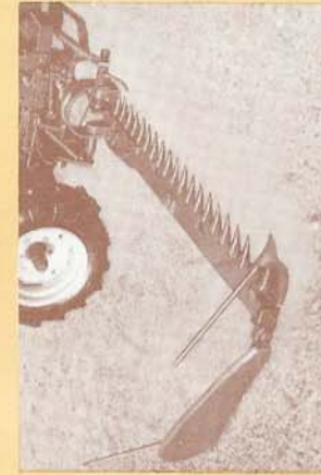
CUTTER BAR: Side mounted 39" cutting bar. Precision built and balanced for minimum vibration. Automatically adjusts to contour of land.
