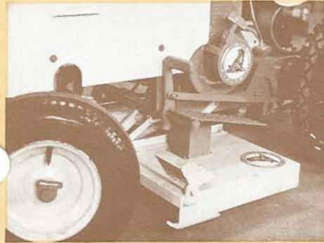
Gear driven, 32 inch cut, twin blades. Direct drive from engine with separate clutch.
